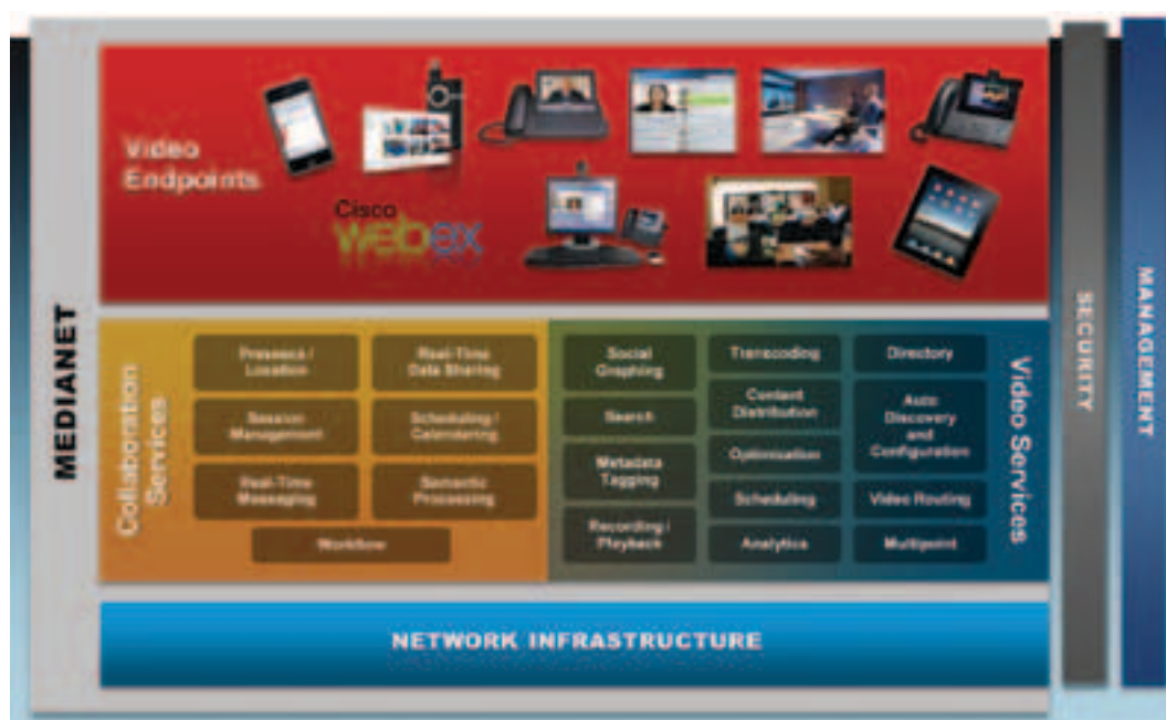
Fig 1. Cisco's Enterprise Video Medianet Architecture
